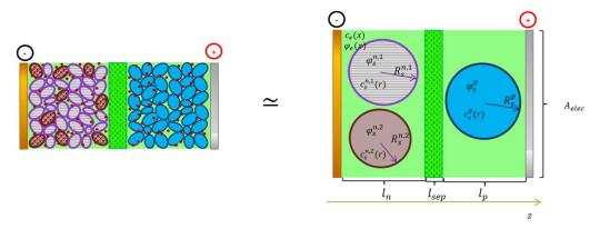
Figure 17: Single Particle Model with electrolyte (SPM-e)
