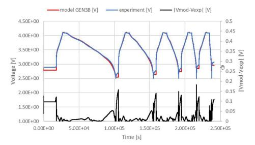
Figure 18: Comparizon between model and experiment on a Crate discharge cycle at 25°C
