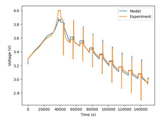
Figure 35: comparizon of model and experiments on HPPC tests
