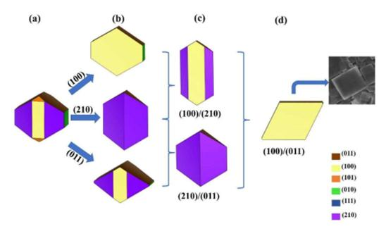
Figure 31: Different morphologies of  $\beta$ -Li3PS4 nanocrystals obtained by varying the relative stability of the various surfaces
