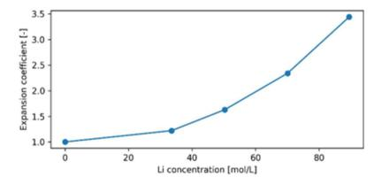
Figure 4: Nonlinear dependency of the volumetric expansion with the Li concentration in LixSi.
