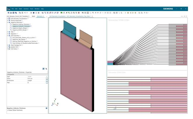
Figure 24: Interface of the 3D cell design simulation template in Simcenter STAR-CCM+
