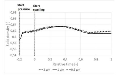
Figure 11: impact of binder properties on particle density
