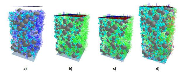
Figure 9: Evolution of the simulated negative electrode material (Graphite: grey, silicon Oxyde: light blue, unbounded contacts: blue, intact bounds: green, broken bounds: red
