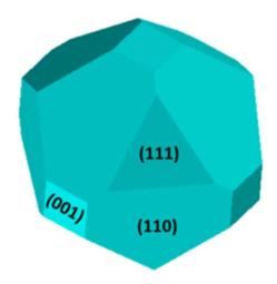
Figure 30: Wulff's polar plot for cubic symmetry of argyrodite
