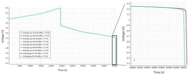
**Figure 37** Charge-Discharge cycle for Gen4 batteries with varying prescribed pressure  $p^{prs}$ . The macrohomogeneous hydrostatic pressure is used to describe the contact factor,  $\gamma$ .
