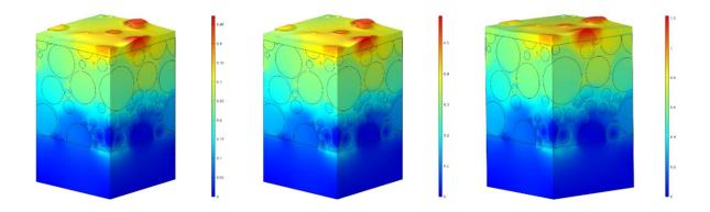
Figure 15: Displacement ( $\mu m$ ) of composite electrode with under volume fraction of LixSiy equals to 0.044, 0.060 and 0.128
