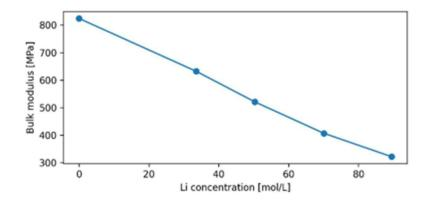
Figure 5: Bulk modulus (in kbar) of LixSi phases vs. their Li molar fraction.
