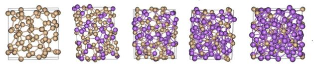
Figure 3: Final unit cell structures for, from left to right: Si, Li0.5Si, Li1Si, Li2Si, Li3.75Si (Si:brown, Li:purple).
