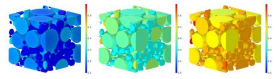
Figure 12: State of lithiation (SOL) at 0.1h, 0.3h, and 0.5h (from left to right)
