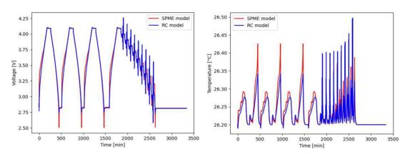
Figure 22: comparizon of the equivalence circuit model (RC) with the SPM-e model
