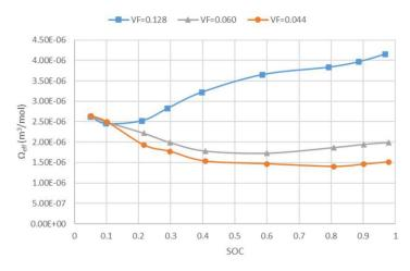
Figure 14: Partial molar volume of lithium in Si-base particles under different volume fraction of LixSiy equals to 0.044, 0.060and 0.128
