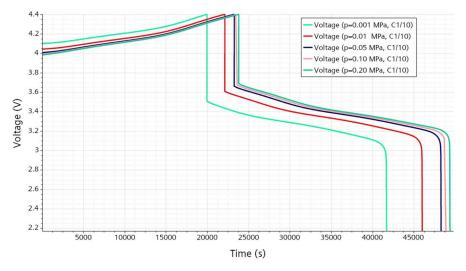
**Figure 36:** Charge-Discharge cycle for Gen4 batteries with varying prescribed pressure  $p^{prs}$ . The prescribed pressure is used to describe the contact factor,  $\gamma$ .
