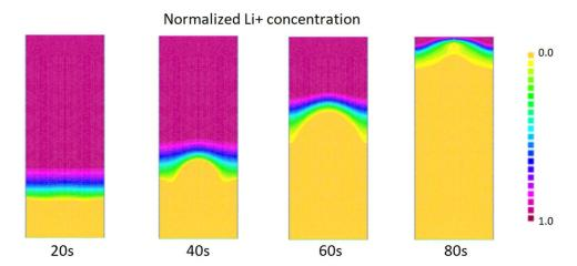
Figure 33: Snapshots of Li metal  $\xi$ , electric potential  $\phi$  and concentration of ion  $Li^+$  at various evolution times
