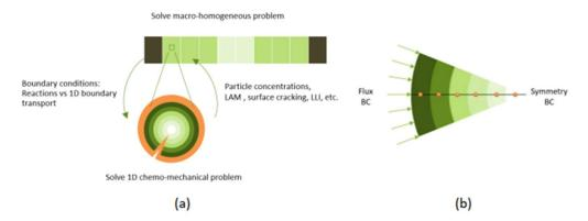
Figure 25: Scale bridging in the sub-grid particle model(a) 1D discretization of the particle model(b)
