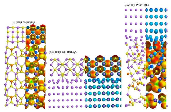
Figure 32: Final optimized interfaces and their charge distribution on the isodensity surface: (a) (100)LPS/(110)Li2S, (b) (110)Li2S/(110)Li-metal, and (c) (100)LPS/(110)Li-metal
