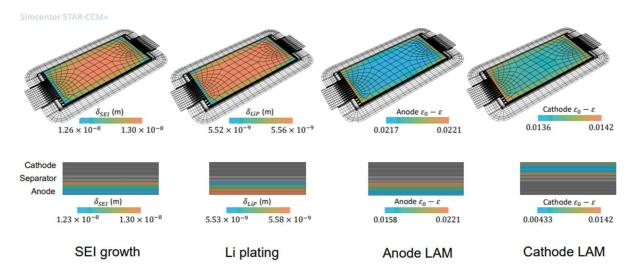
Figure 27: Heterogeneous aging in cathode and anode: in-plane and in thickness direction
