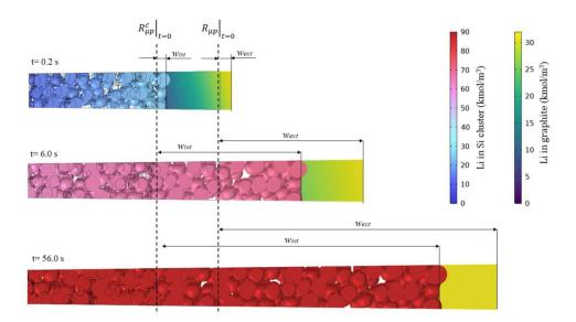
Figure 7: Intercalation-driven deformation. The progressive increase in Li concentration in graphite and silicon clusters forces the inner and outer shell radii to expand. The figure refers to the configuration with a 0% conversion rate.
