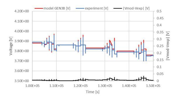
Figure 19: Comparizon between model and experiment on a window of a HPPC cycle at 40°C
