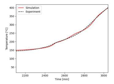
Figure 23: Modeled and experimental cell temperature comparison during self-heating phase
