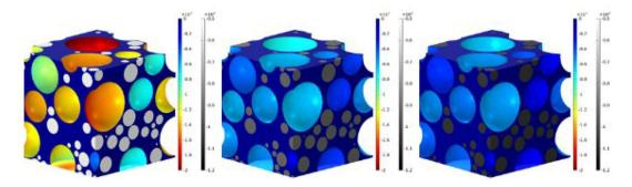
Figure 13: Local current density (mA/m2) of graphite and Si-based particles at 0.1h, 0.3h, and 0.5h (from left to right)
