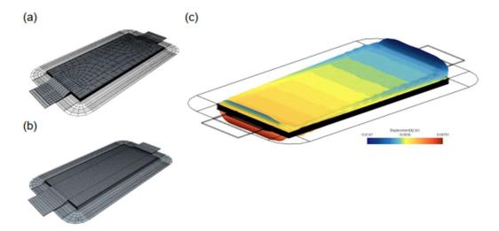
Figure 26: V-FE discretization overlay(a) FE discretization (b) Swollen configuration of the thermo-mechanical FE simulation (c)
