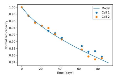
Figure 20: normalized capacity loss during calendar aging compared to experimental data
