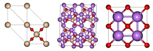
Figure 2: Unit cell structures for SiO2, Li4SiO4 and Li2O (Si:brown, Li:purple, O:red).
