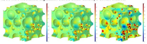
Figure 16: Pressure (GPa) endured in binder-electrolyte with under volume fraction of LixSiy equals to 0.044, 0.060 and 0.128
