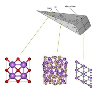
Figure 6: Representation of the spherical wedge used to perform the mechanical simulations. (Si:brown, Li:purple, O:red)
